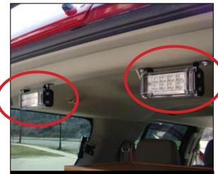
We've Got Your Back.... two single lights mounted to the rear headliner provide bright rear warning power in the rear window of a 2008 Ford Expedition.
